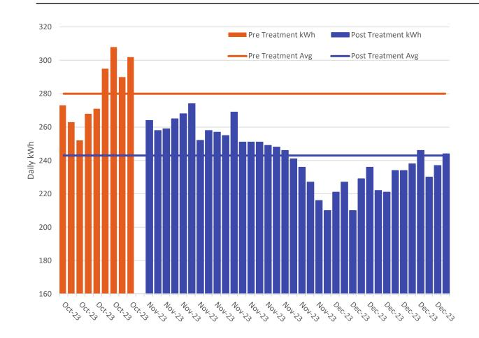
This chart shows a self-storage facility's daily energy use of an entire level's air conditioners. Comparing normal usage (orange) with reduced usage post-ThermaClear® implementation (blue).
